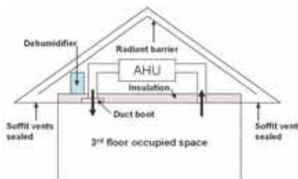
Figure 5: Diagram of modifications needed to “seal attic and install a dehumidifier.”
