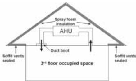
Figure 4: Diagram of modifications needed to seal attic and insulate at roof.
