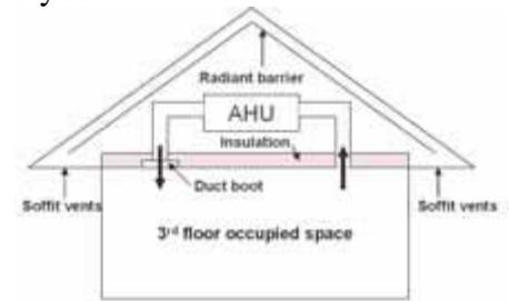
Figure 1: Diagram of attic and HVAC system components at time of inspection.
