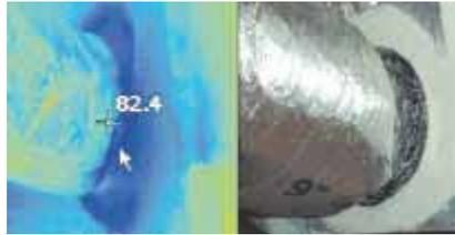
Figure 3: Thermal image (left) and visible light image of plenum to flex duct connection. Note significantly colder surfaces where duct insulation is compressed.
