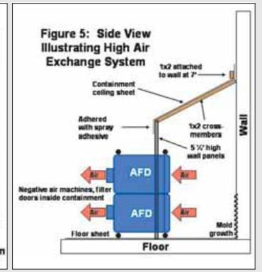
Figure 5: Side View Illustrating High Air Exchange System
