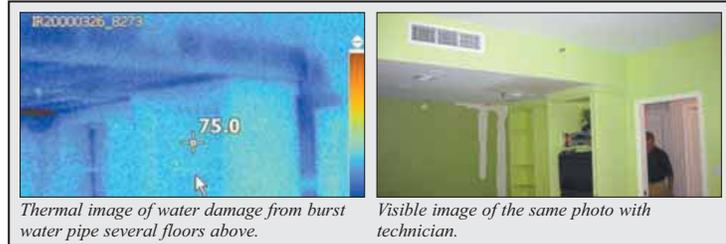
Thermal image of water damage from burst water pipe several floors above. Visible image of the same photo with technician.
