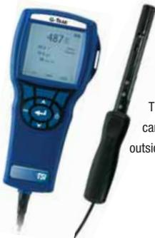
The TSI Q-Trak Indoor Air Quality Monitor can measure ventilation effectiveness and percent outside air to run your system at maximum efficiency.
